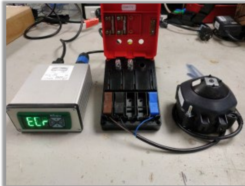
Pictured: Uniprogram connected to CLIFF Electronic Components Quicktest power tester and a Wellington ECR motor.
