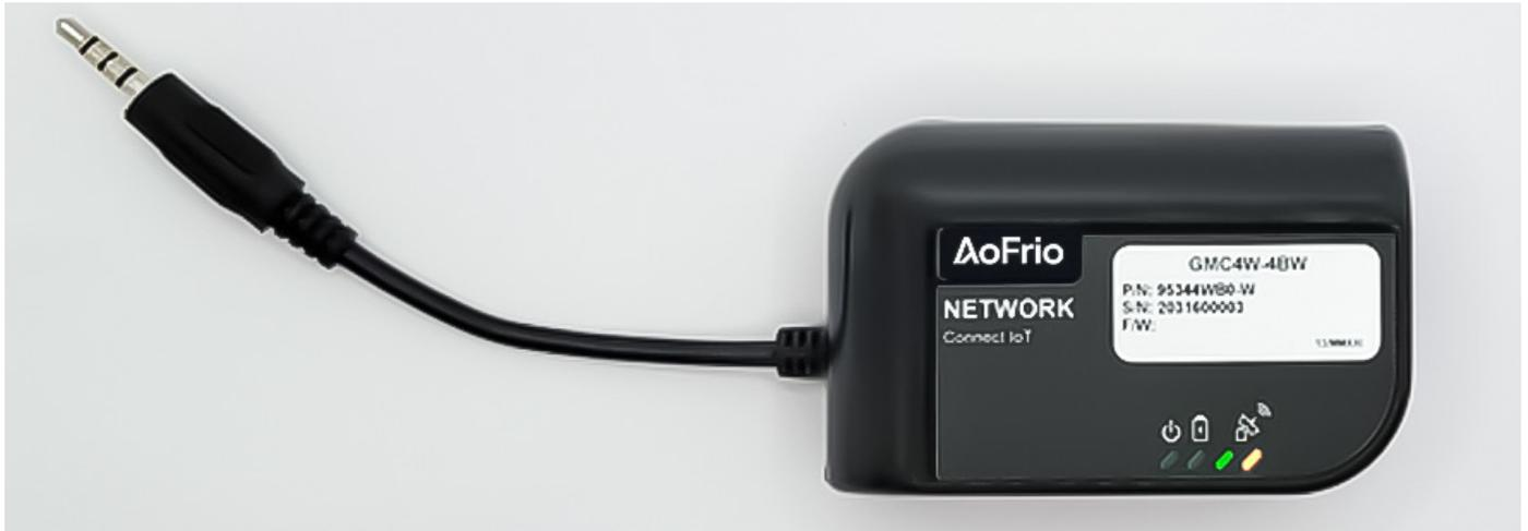
1. Plug the 3.5mm connector from **Network Pro** into the supplied cable.
